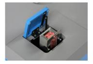
Put the cell into the InfraLUM FT-12 analyzer, choose the analyzed product in the menu, and start the measurement
