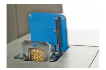
Fill the sample cell, place it into InfraLUM FT-12, choose the analyzed product in the menu and start the measurement.
