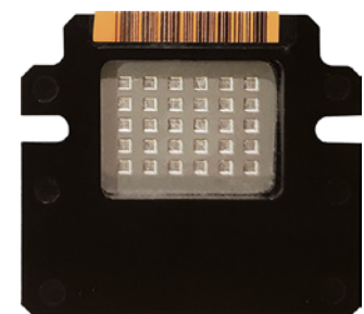
Aluminum microchip with 30 microreactors
