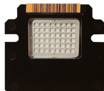
Stainless steel microchip with 48 microreactors.
