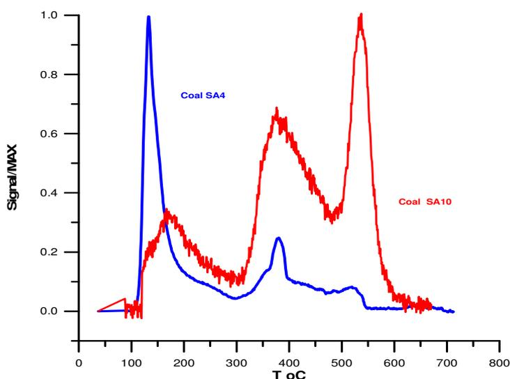
The low-temperature peaks can be attributed to mercury bound by physical sorption and occluded, whereas the mid- and high- temperature peaks to mercury bound to organic coal matrix, sulfides, and silicates. The technology enables identifying mercury bound to pyrite and other sulfides. The thermoscaning technique gives additional information about mercury speciation in samples.
