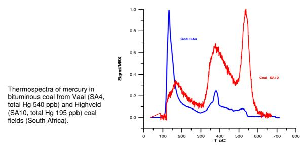
The low-temperature peaks can be attributed to mercury bound by physical sorption and occluded, whereas the mid- and high- temperature peaks to mercury bound to organic coal matrix, sulfides, and silicates. The technology enables identifying mercury bound to pyrite and other sulfides. The thermoscanning technique gives additional information about mercury speciation in samples.
