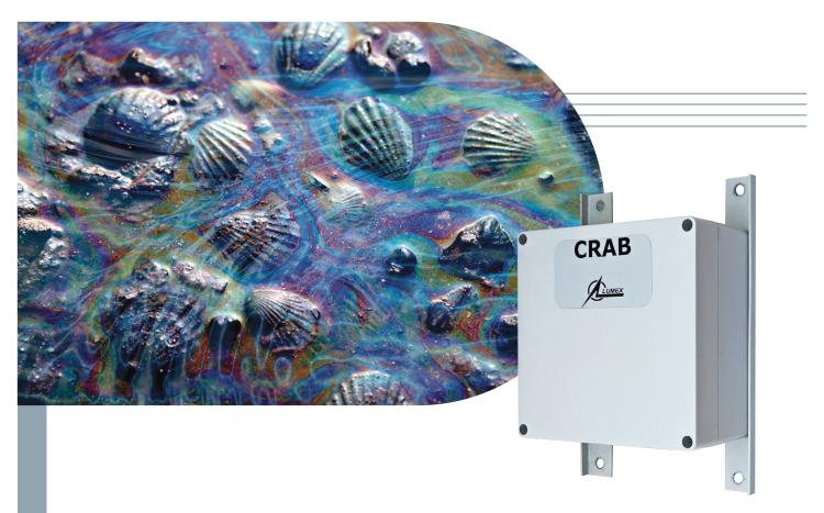
CRAB is an easy-to-operate, active optical sensor of the water surface oil slicks. The instrument detects the presence of oil using laser sensing with a vertical spot light beam and measuring the differences in the reflection properties of water and oil products.
