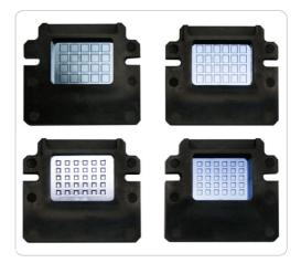
Disposable microchips in different microreactor formats and materials: silicon microchips with 20, 24, 30 microreactors; aluminum microchip with 30 microreactors.
